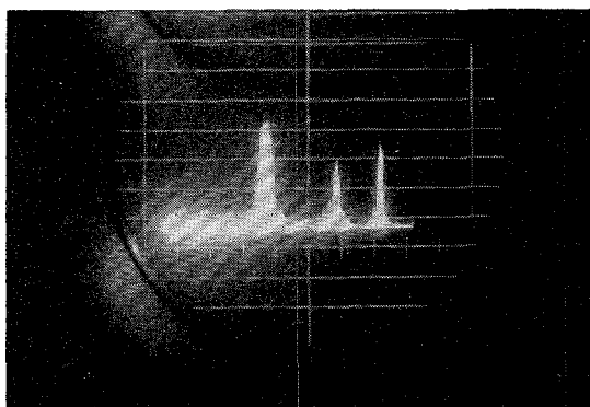
Fig. 6—Spectrum of 2 \mu sec of storage between preferred frequencies using waveguide delay line.
